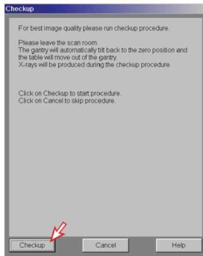
The automatic check-up procedure executes a set of functions to ensure that the CT scanner is well conditioned and is able to provide high quality images.
